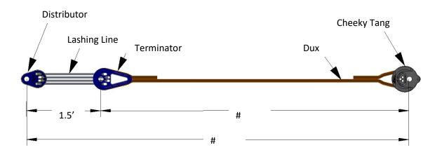
Through Hole dia. = # Mast Thickness = #
